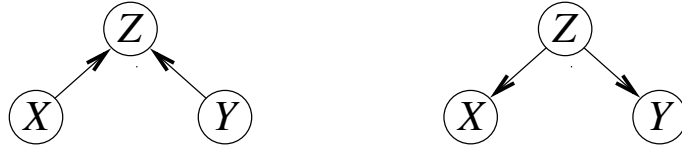
Figure 2.5: In the left directed graphical model, X and Y are marginally independent of each other, but became dependent when conditioned on Z , i.e. X \perp\!\!\!\perp Y but X \not\perp\!\!\!\perp Y|Z . In the right directed graphical model, X and Y are conditionally independent of each other when conditioned on Z , but they are not marginally independent.
