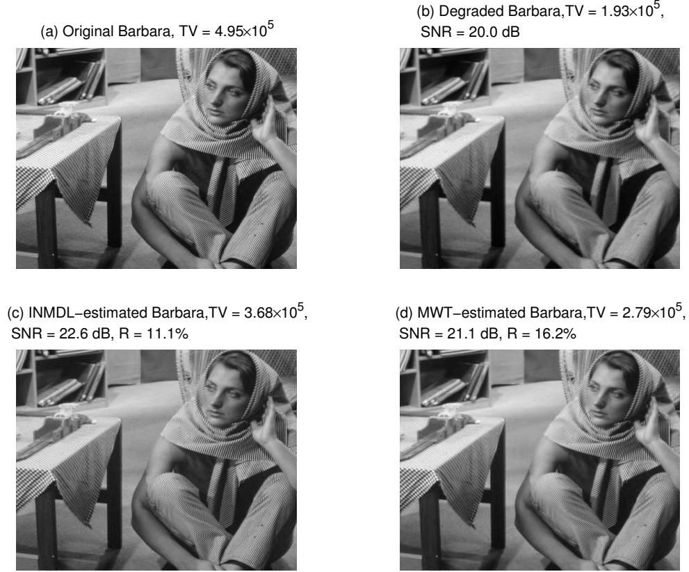
FIGURE 1. Comparison of estimator performance for INMDL and the MWT algorithms on 8-bit grayscale test image barbara with N = 512 \times 512 . The noise variance is \tau^{-1} = 1.0 and the lowpass filter used to degrade the image was: \cos^{p_x} \left( k_x \pi / \sqrt{N} \right) \cos^{p_y} \left( k_y \pi / \sqrt{N} \right) in the Fourier domain with p_x = p_y = 3.0 . TV denotes the total variation (240) and R is the fraction of nonzero wavelet coefficients in the estimate. The GGD shape parameter was estimated by the INMDL-algorithm to: \nu = 0.606 .
