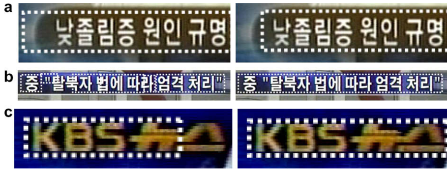
Fig. 11. Representative results of the text line refinement. Left: initial localized text line. Right: refined text line. (a) Text boundary shrinking function. (b) Text boundary combination function. (c) Text boundary extension function.
