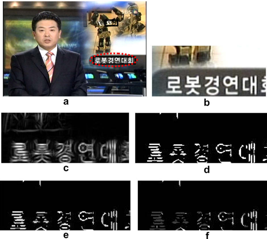
Fig. 5. Features extracted by a stroke filter in a real text image. (a) Original image. (b) Text sub-image. (c) Stroke response map. (d) Binarization of (c). (e) Stroke width map. (f) Stroke orientation angle map.
