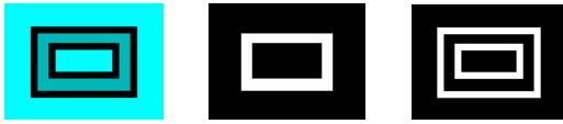
(a) Source image (b) Bright SF resp. map (c) Dark SF resp. map Figure 5. Bright and dark stroke filter (SF) response maps.
