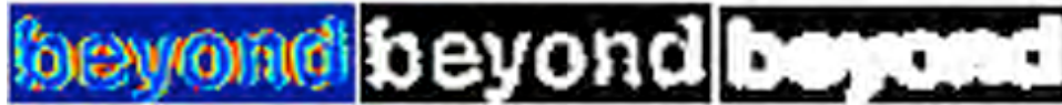
Fig. 9. Phase of the vertical filter multiplied by the mask issued from the text extraction (left) and result after global thresholding (middle). Improvement is obvious from the binary version (right).
