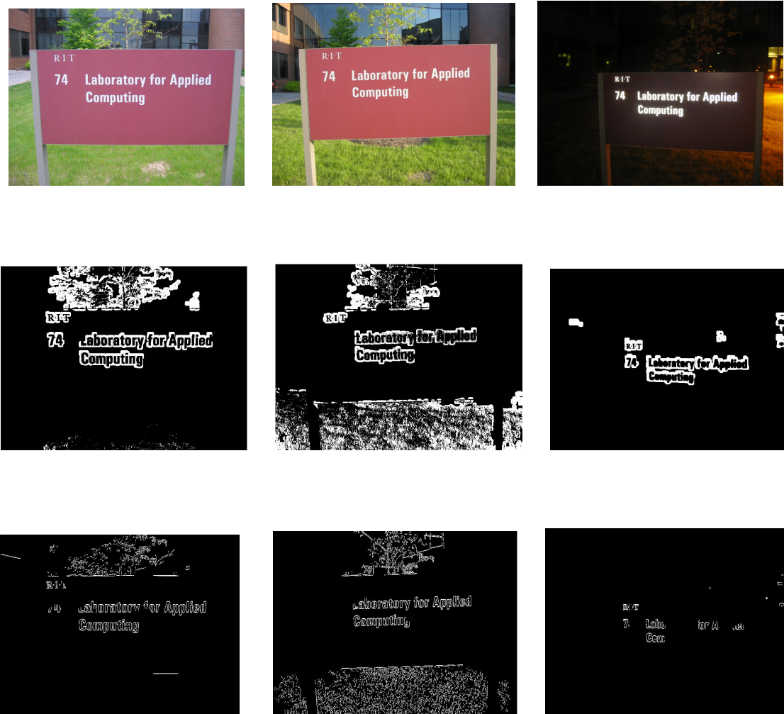
Figure 18. (Row 1) Original images at three different lighting conditions (Row 2) Results from edge based algorithm (Row 3) Results from connected component based algorithm
