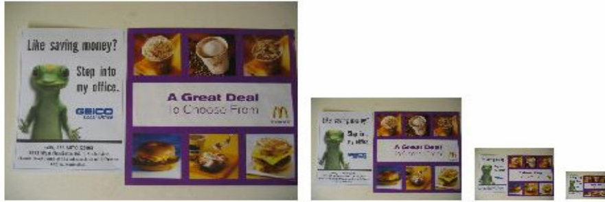
Figure 3. Sample Gaussian pyramid with 4 levels
