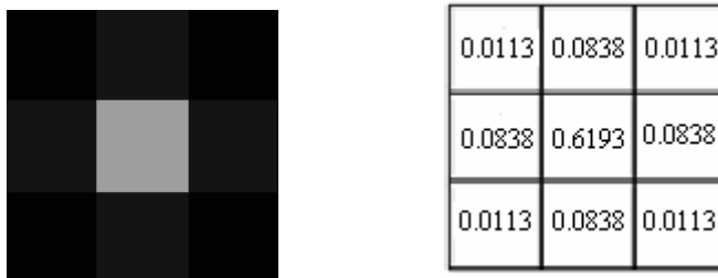
Figure 2. Default filter returned by the fspecial Gaussian function in Matlab.
